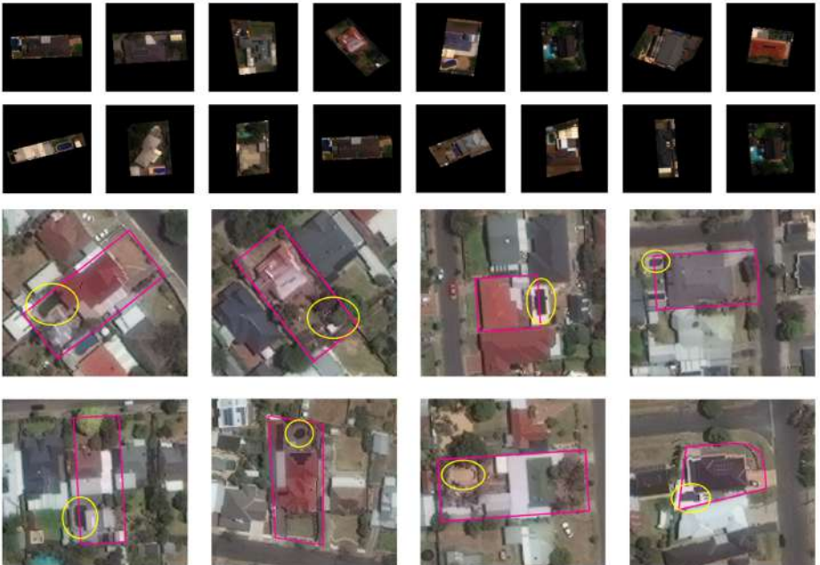
Figure 8. Sample image “chips” (top) are fed into the machine learning algorithm to teach it automated object identification in satellite imagery (bottom). Individual properties are outlined in pink and swimming pools are marked by yellow ellipses. Satellite imagery, 2019, courtesy of DigitalGlobe, a Maxar company.
