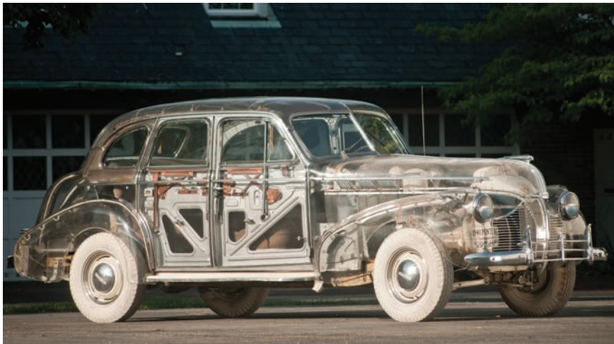
FIGURE 5 The Pontiac Deluxe Six, "Ghost Car" with a plexiglass body produced by Rohm and Haas for the 1939 World's Fair in New York.
