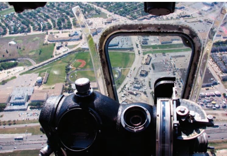
FIGURE 2 nose of the plane. Note the lack of wavy distortion in the triangular section in the center, and the effect of the distortion on the rest of the material.
